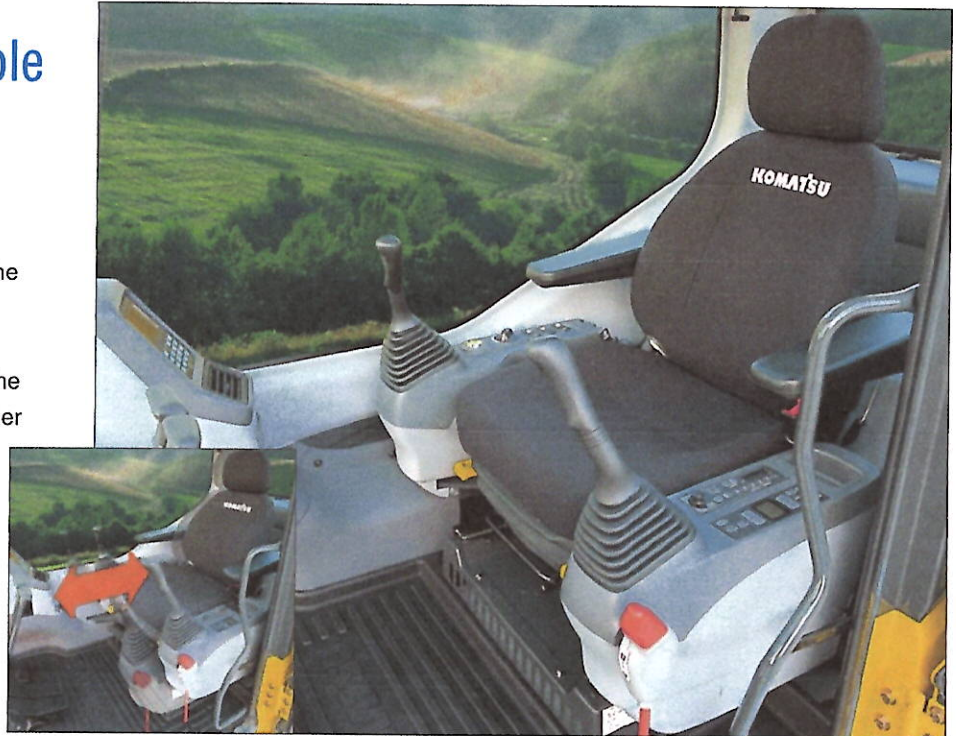
Seat Sliding Amount: 340 mm 13.4", increased 120 mm 4.7"
