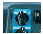
Auto High: High mode provides maximum rim pull and fast cycle times by shifting the transmission at high engine speeds. This mode is suitable for hill-climb and load and carry operations.
