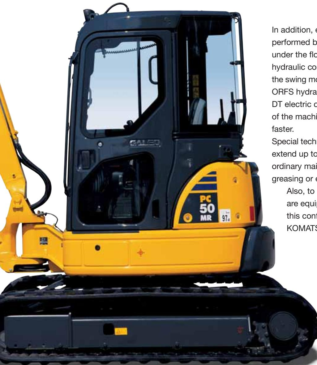
In addition, extra-ordinary maintenance can be performed by simply tilting the cab upwards: under the floor, the operator can find all major hydraulic components, like the main valve or the swing motor.
