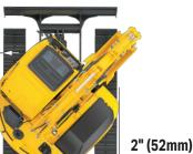
Protrusion from the track (Frame)
