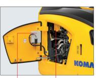
Washer tank Auxiliary hydraulic circuit return filter
