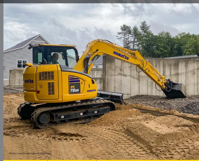
**NET HORSEPOWER** 68 HP @ 1,850 rpm 51 kW @ 1,850 rpm
