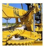
Lift system provides widest lift cylinder stance of any grader for maximum stability and reduced end-to-end blade interaction, resulting in better fine grade control.
