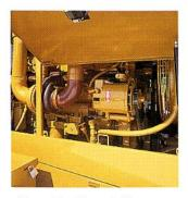
Job-matched dependable Cummins diesel power offers superior fuel efficiency as the engine's peak torque is matched to transmission shift points. Optional side panels are lockable and provide easy access for routine maintenance.
