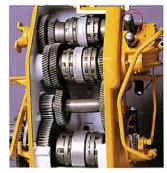
The exclusive **Champion 8400** grader transmission is now in service in more than 10,000 units. Evenly proportioned gear ratios provide precise, job-matched speeds for any grading application. A new "Smart Shift" feature lets the operator easily customize shift patterns to the job at hand.
