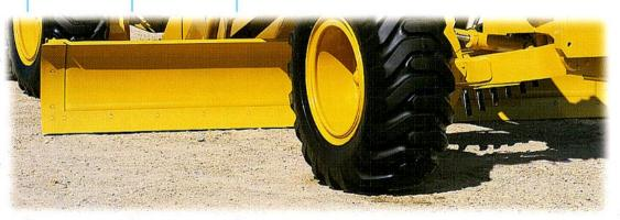
With its 72° front axle steering arc, Series IV moves comfortably in confined work areas. The tight turning radius means faster finishing in culde-sacs and less following-up in the corners.
