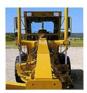
Sloped frame for increased forward visibility. First user life time frame warranty on the front and rear frame sections.
